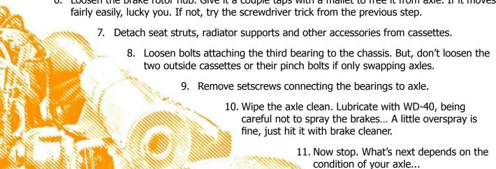
TOTALLY FINE, JUST MAKING A **SWAP FOR TUNING PURPOSES:** Carry on, just take care not to crowbar the bearings out of alignment with the axle as you remove it... especially after it's free of the first bearing.
